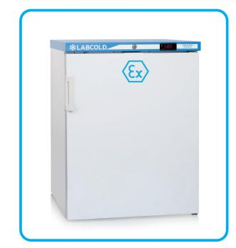
The **Labcold** ATEX freezer range has been designed with an interior which is licensed as a Zone 2 hazardous area under 2014/34/EU (ATEX Directive) in order to store products which are classed in explosion group IIB+H2 and temperature class T6 under 2014/34/EU (ATEX Directive).
